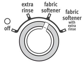
This washer has been designed to allow the use of a fabric softener dispenser ball, which you will need to purchase. Always follow the manufacturer's instructions for correct instructions on how to use the dispenser ball. Then select the Fabric Softener option. The fabric softener dispenser ball will release the fabric softener during the rinse cycle.
